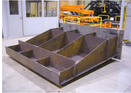
Steel Deck Test Section Fabrication
